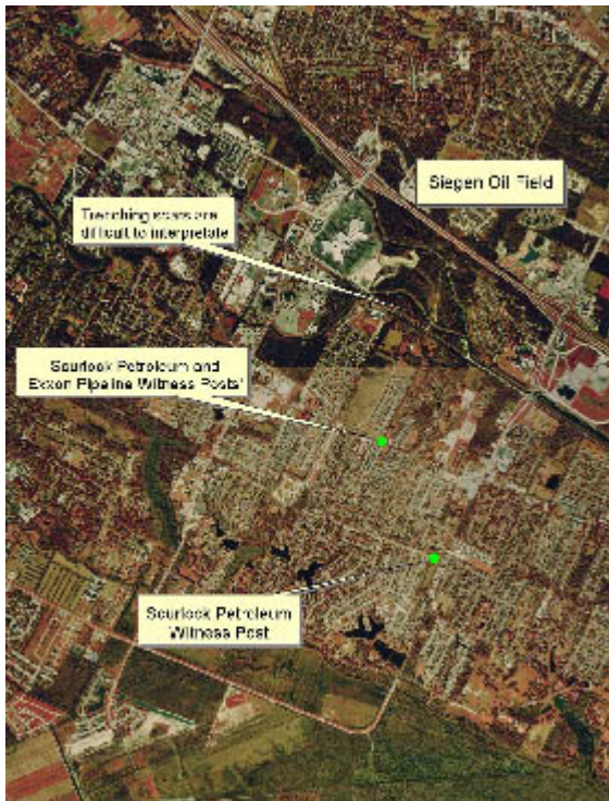
Figure 10. Untraceable pipeline witness posts.
